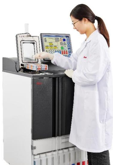
*The new ASP6025 S includes magnetic stirrer technology designed to optimize paraffin infiltration performance, helping reduce processing time and enhancing reagent exchange within the tissue cells.*
