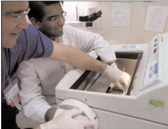
We then turn the cryostat wheel continuously, without any hesitation, and catch the sections with the brush. This precise, delicate motion can be compared to catching a falling snowflake with the brush. In order to do this, the brush must continue to move in an elliptical motion, which in conjunction with the right hand turning the wheel is like turning the pedals of a bicycle. I have found that the best way to teach this skill is to hold hands.
