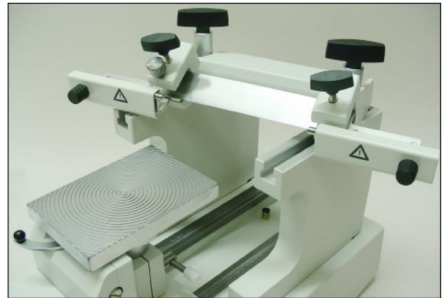
Fig. 5 Large (90 x 130 mm) specimen stage
