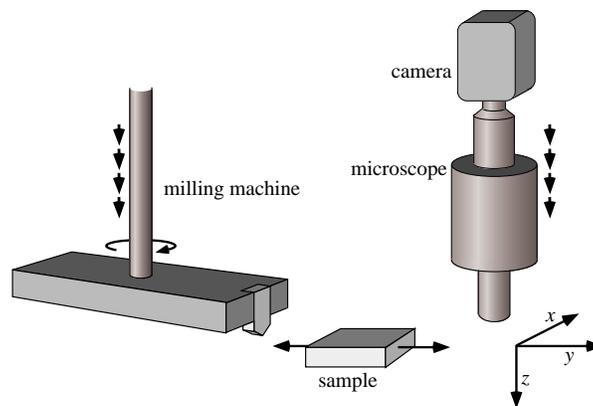
FIG. 3. Schematic drawing of the serial sectioning procedure. The sample translates from the miller to the microscope in the  $y$ -direction. The sections are taken in  $z$ -direction. The two lines of four short arrows indicate the simultaneous movement of the miller and microscope in  $z$ -direction between the individual cuts.
