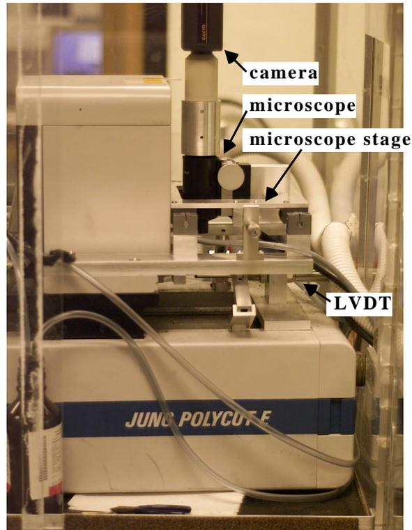
FIG. 2. Attachment to the micromiller to make serial sections
