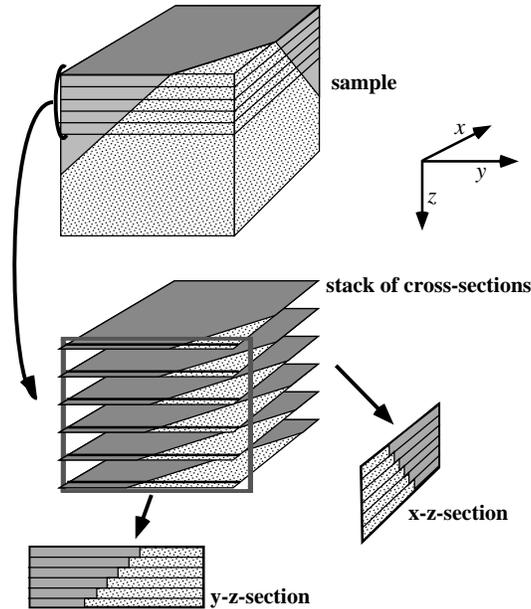
FIG. 7. A cube of aluminum and mounting material with a flat but tilted interface between the materials is sectioned. From the sections an  $x$ - $z$ - and an  $y$ - $z$ -cross-section can be extracted.
