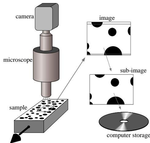
FIG. 4. Microscopy of the surface. The image of a section of the sample surface is captured. A sub-image is then created based on the position information given by the LVDT (see text) and saved to disk. The large arrow at the end of the sample denotes the direction of translation.
