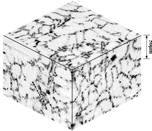
FIG. 10. Reconstructed Al-Si alloy. The bright phase is aluminum and the dark phase is silicon. The microstructure shows aluminum dendrites and a aluminum-silicon eutectic phase. Shown is a tilted view of a reconstructed volume. The upper area is one of the original cross-sections. The two sides are the  $x$ - $z$ - and  $y$ - $z$ -sections that were reconstructed from the data set.
