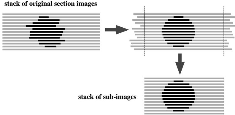
FIG. 5. A set of perfectly aligned sub-images can be obtained from a set of images from the different sections if the displacement between the different sections is known
