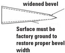
The new, or factory reconditioned, Leica Knife has very precise wedge and cutting facet angles. These angles permit the knife to „meet“ the glass hone plate in the correct manner for proper coarse and fine honing.
