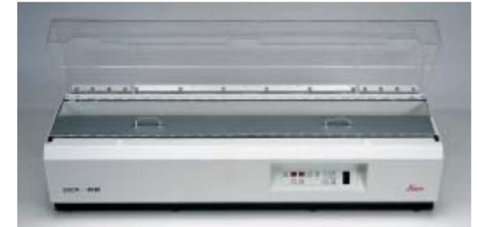
To prevent evaporative reagent loss when not in operation, the staining track can be covered with the included reagent lids.
