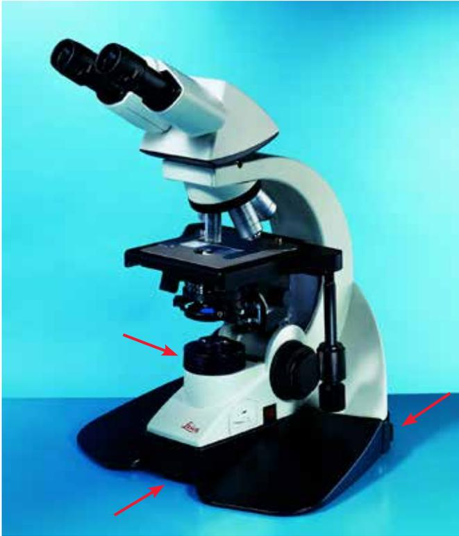
**Figure 2:** The optional Ergolift accessory underneath the microscope alters the distance from bench to eyepieces, which is particularly useful for tall users. The adjustment wheels (red arrows), enable the height to be varied between 40 and 80 mm, and for the microscope to tilt up to 17mm +/- 1mm. Hands and forearms rest comfortably on the skin-friendly surfaces on both sides.
