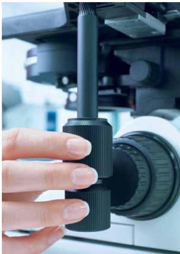
**Figure 7:** One hand operation of focus knob and stage drive with DM3000 microscope.
