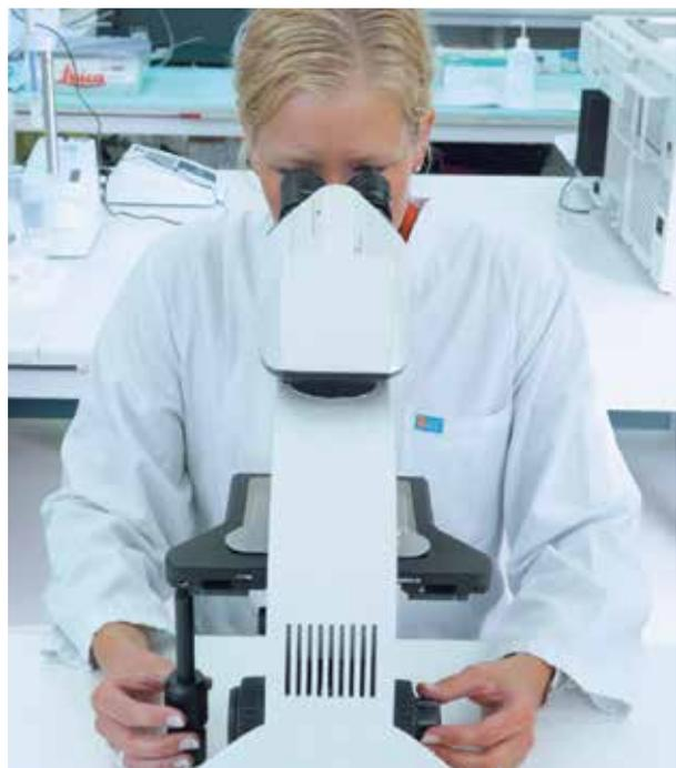
**Figure 5:** Optimal ergonomic operation of a microscope thanks to symmetrical layout of coaxial drive and focus knobs. Shoulders are level, the spine is straight and arms are resting at a comfortable angle without stretching.
