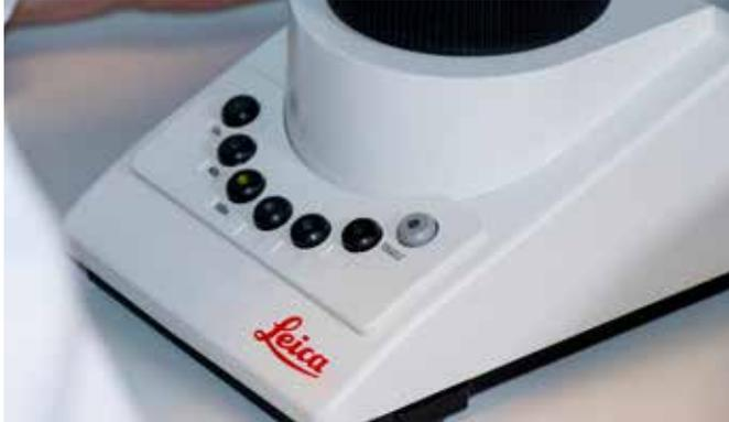
Figure 8: Control buttons for objectives and toggle mode with DM3000 microscope.
