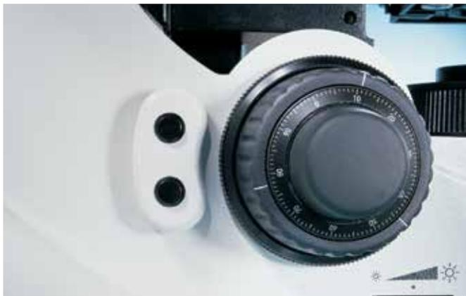
Figure 9: Freely programmable buttons behind each focus knob (DM3000 microscope).
