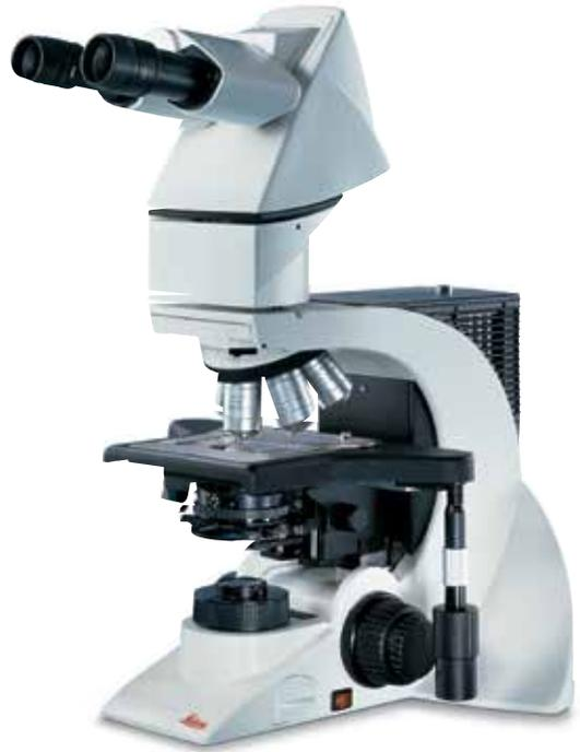
**Figure 6:** Left: A telescopic ergomodule between stand and observation tube allows for easy adjustment of the microscope height enabling to frequent changes to the user's working position or to facilitate multiple users employing the same microscope, without forfeiting ergonomics.
