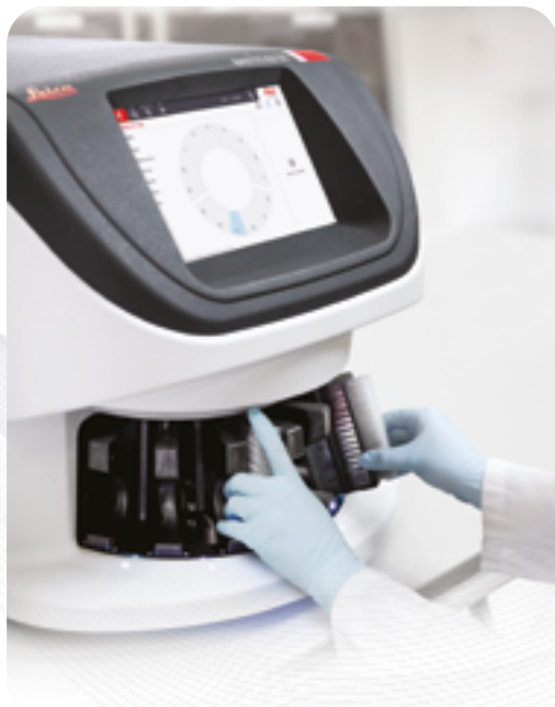
Aperio GT 450 DX open face design allows you to continuously load racks while scanning is in progress to maximize productivity.
