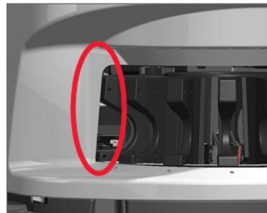
2. Ensure the racks in the rack loading area are inserted correctly:
