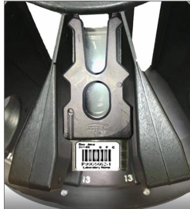
3. When you insert the rack, ensure the rack position and the rack status light turns light blue (waiting to scan):
