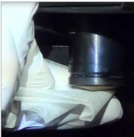
7. With a clean lint-free microfiber cloth, use the same technique described in step 6 to clean the Koehler. The Koehler is located below the objective, as shown circled in white below.
